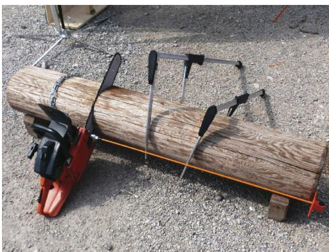
Figure 7. Consistent length firewood rounds are made easy with the Nestle Kolibri chainsaw attachment.
