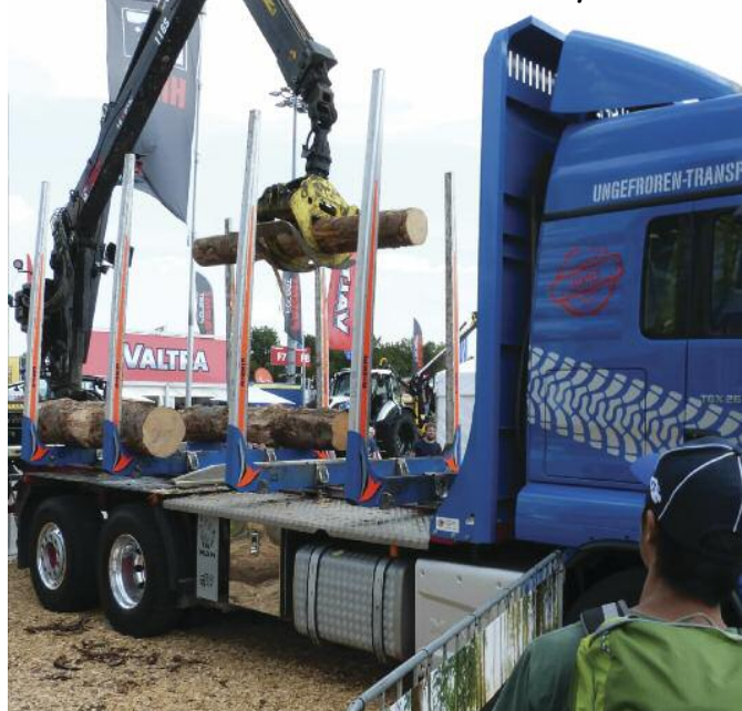
Figure 6. Hiab HiVision remote crane operation system allows the operator to stack from the cab for increased safety and comfort.
